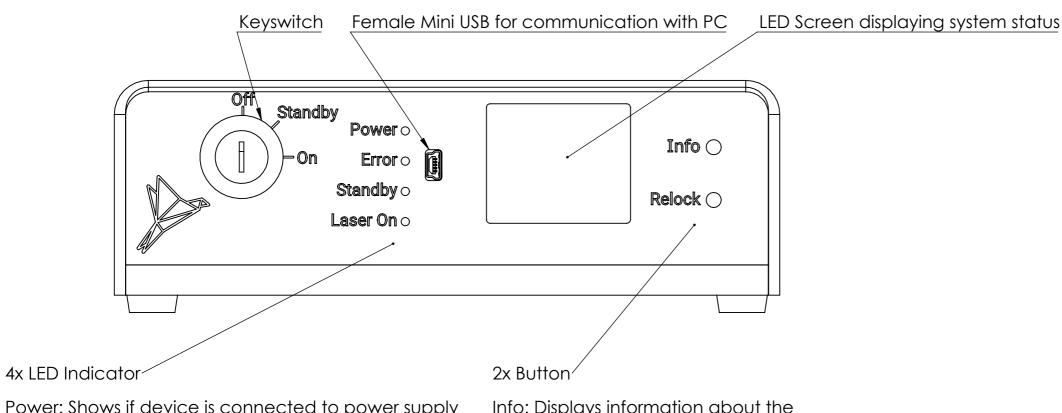
Power: Shows if device is connected to power supply Error: Indicates an error in the system Standby: Indicates device is waiting for a command Laser On: Indicates laser diode being active
