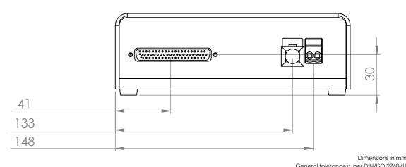
General tolerances: per DIN/ISO 2768-fH Form/Position tolerances: per DIN/ISO 1101 Edges: per DIN/ISO 6784
