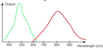
These crystals combine supreme thermal and optical properties with broadest lasing range among other materials. Its indefinite stability and short lifetime, in addition to lasing over entire band of 660 to 1050 nm makes Ti:sapphire lasers suitable for variety of applications spanning from material processing to time resolved and multi-photon
