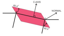
**Brewster-angle cut** is used to eliminate reflection losses, increase polarization contrast, avoid formation of parasitic pulses in ultra-short pulse oscillators or even induce negative dispersion. Brewster cut faces are often left uncoated in order to increase damage threshold of the surface.
