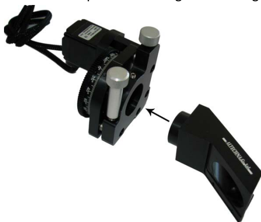
Fig. 1. Assemble the mechanical part of attenuator.
