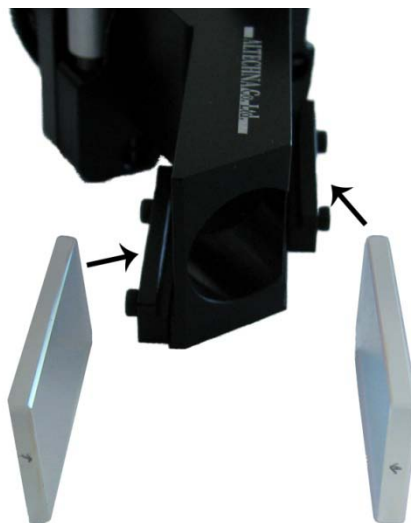
Fig. 5. Place the polarizers and fix them with the clips. ( Please note that arrows on the sides of polarizers must face each other)
